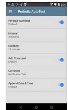
Periodic AutoTest enables monitoring infrastructure for intermittent issues
